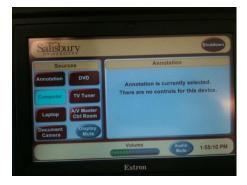
When a source is chosen, its corresponding controls appear on the right side of the touch screen, if applicable.
