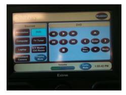
Program audio control is on the left side of the main page. Rooms with microphones have additional audio controls, which can be used to mute, unmute and adjust the microphones. Tap the **Audio Controls** button to access these additional controls.
